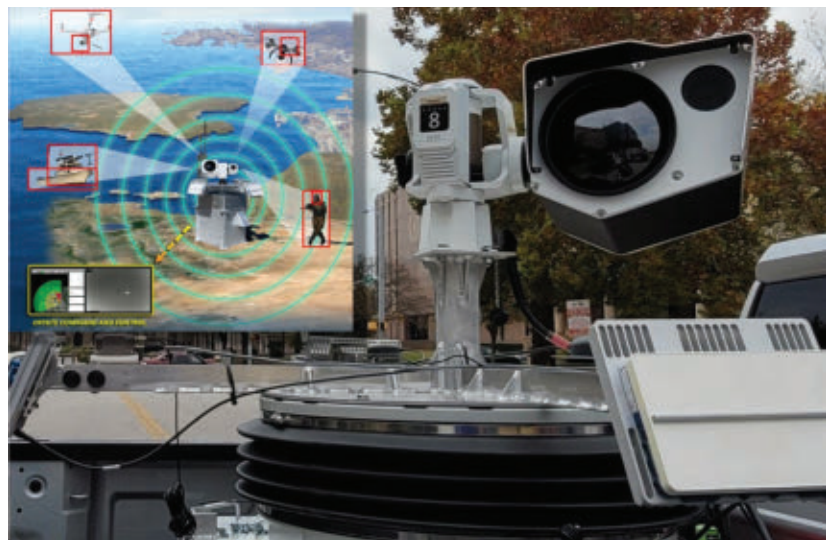
▲ Threat Tracker is an autonomous threat detection system developed by a small team of engineers and scientists at the Coastal and Maritime Security branch at Naval Surface Warfare Center Panama City Division. Threat Tracker is an autonomous, multi-platform threat detection system that uses radar and sensor technologies coupled with video analytics and machine learning algorithms to detect, track and classify potential threats. U.S. Navy illustration.
